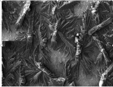
Figure 2. Photo shows large crystals with voids in the phosphate coating.
